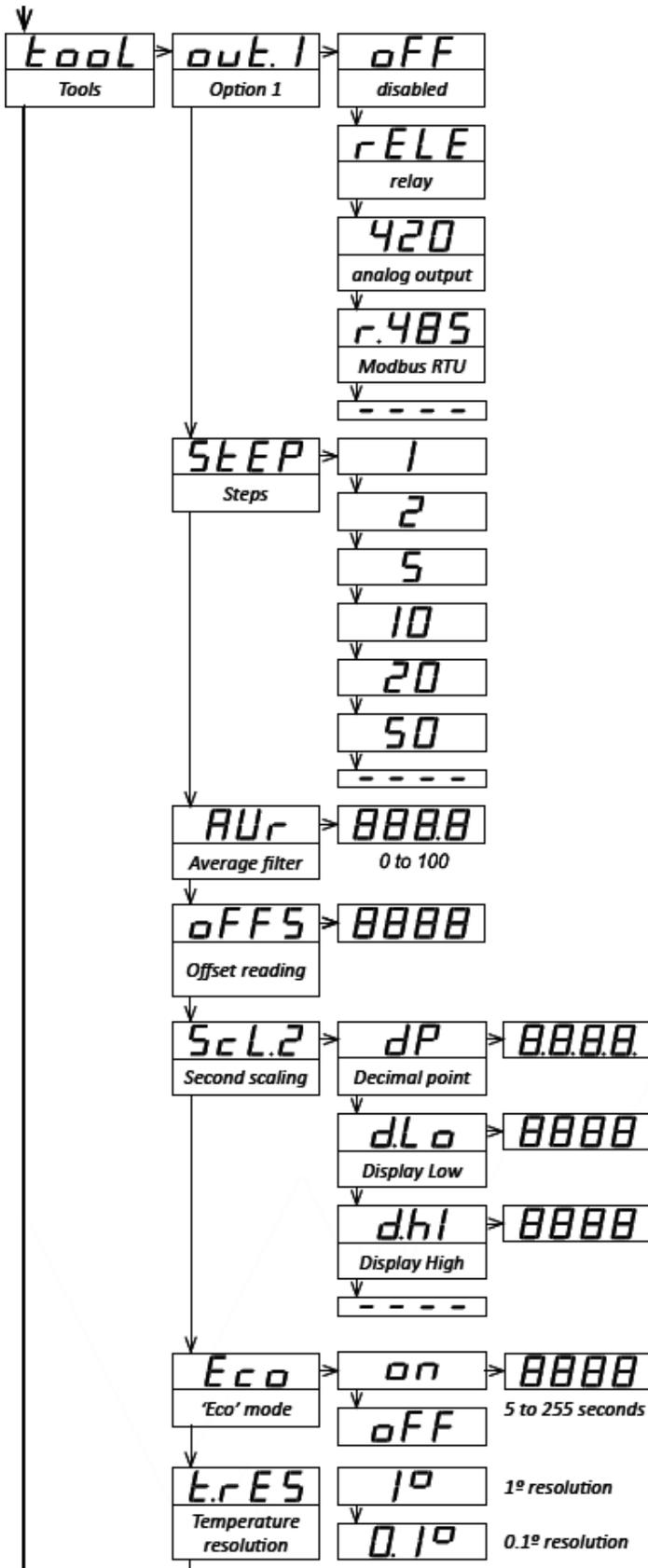
The **Tools (tool)** menu is used to configure the meter.
