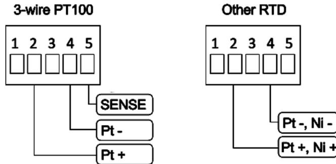
**Provision for lead wire resistance:** A 3-wire connection is jumper selectable with Pt100 RTDs to subtract lead wire resistance. If a 2-wire connection is used, the instrument allows a fixed number of counts to be subtracted from the resistance reading. This is done with the programmable “oPFFS” offset parameter.
