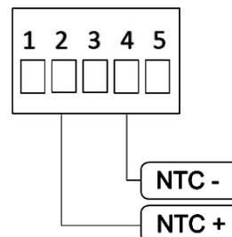
**NTC probe types:** To see if the L40 is compatible with specific NTC thermistor type, check the thermistor data sheet and note the parameters  $R_{25}$  and Beta. The instrument can be programmed for Beta values from 2000 to 5500 and accommodates resistances from 100 P to 100 kP.
