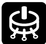
**Potentiometric Signals:** In potentiometric (or pot follower) applications, the L40 applies a 5 Vdc excitation voltage across a 3-wire potentiometer, and the signal to be measured is picked off by a wiper. The reading is in percent and is not affected by changes in excitation voltage. This technique is commonly used to measure linear or angular position.
