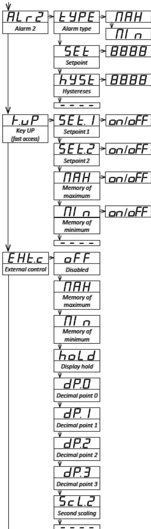
**The Fast Access (K.up) menu** allows specific functions to be accessed by pressing the Up ▲ key. Select “on” to select a function for fast access, “off” to deselect. Super-fast access is provided when only a single function has been selected. Pressing the Up ▲ key will then jump to that function.
