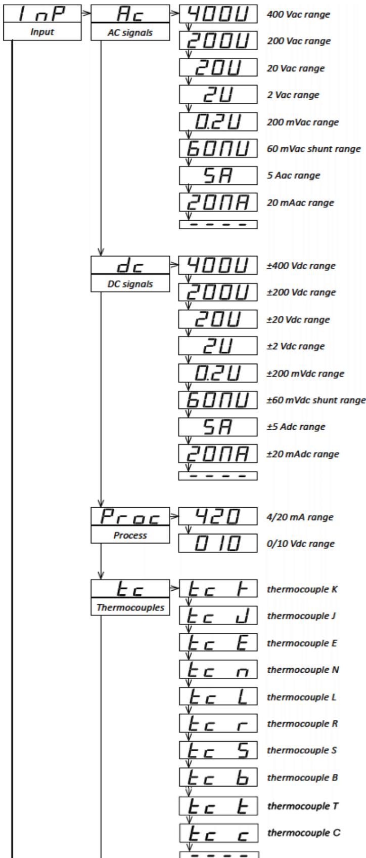
**AC input (Ac).** Select the full scale range. Choices are 400 Vac (factory default), 200 Vac, 20 Vac, 2 Vac, 200 mVac, 60 mVac, 5 Aac, and 20 mAac. AC measurement provides True RMS readings.
