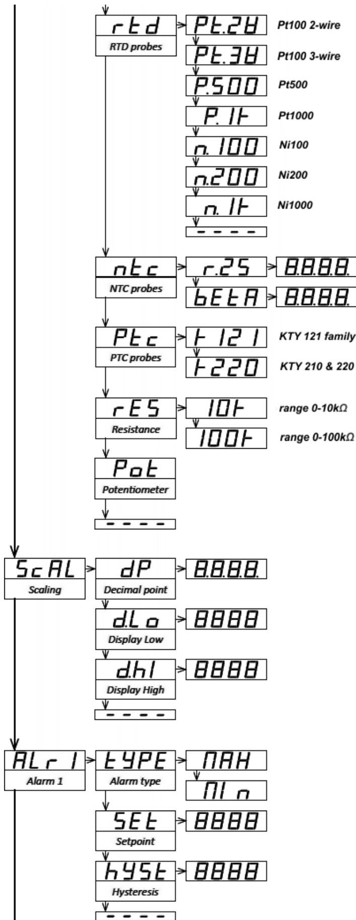
**RTD input (rtd).** Select the RTD type. Use the programmable offset feature (oFFS) to subtract counts for lead resistance.
