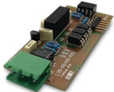
The optional S1 module provides an isolated Modbus RTU serial output. It is installed in Slot 1 and plugs directly into the display board. With only a single function (4 = read register), it is very easy to use.
