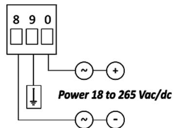
UL 61010-1 requires a 250 mA slow-blow fuse for power > 50 Vac/dc, or a 400 mA slow-blow fuse for power < 50 Vac/dc.
