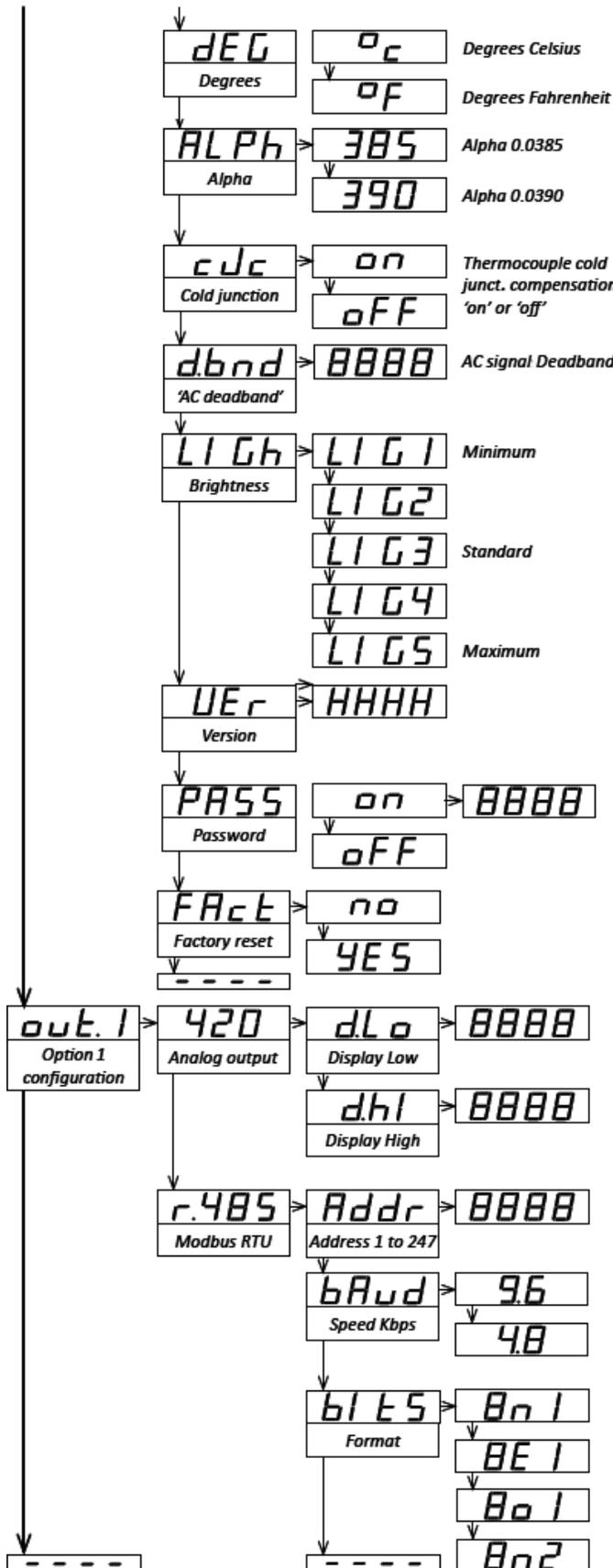
**Degrees (dEG)** allows selection of °C or °F for temperature.
