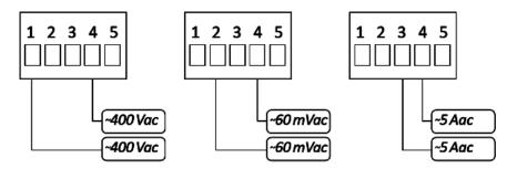
**Display scaling:** AC voltage or current signals can be scaled to produce readings from -1999 to 9999 with any decimal point. The meter's first or second scaling method can be selected using the meter's external control input.
