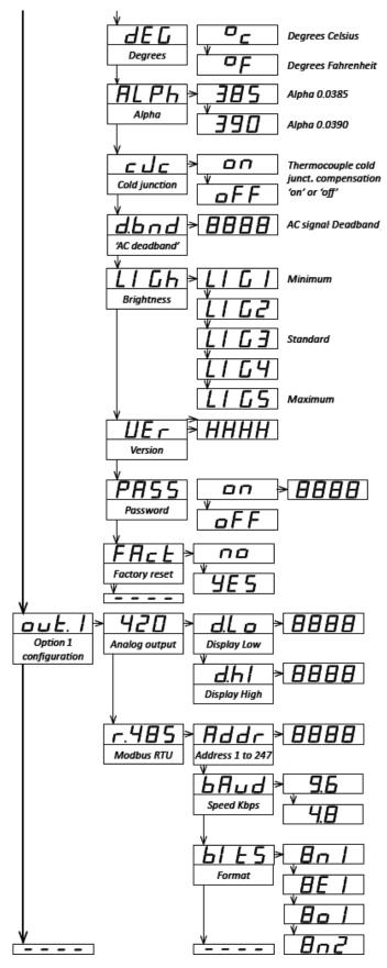
**Degrees (dEG)** allows selection of °C or °F for temperature.
