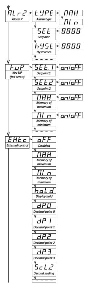
The Fast Access (K.up) menu allows specific functions to be accessed by pressing the Up  $\blacktriangle$  key. Select "on" to select a function for fast access, "off" to deselect. Super-fast access is provided when only a single function has been selected. Pressing the Up  $\blacktriangle$  key will then jump to that function.
