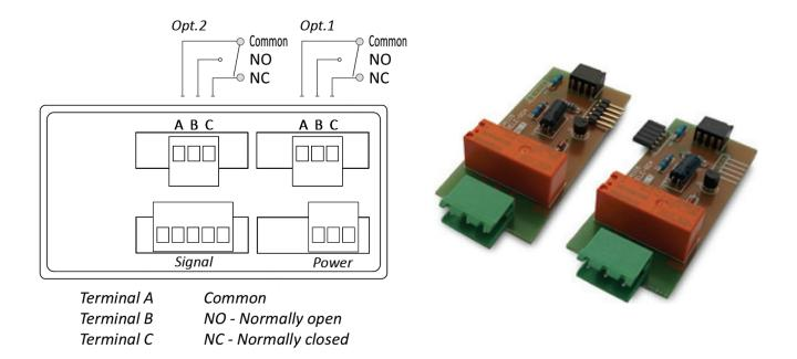
The optional A1 relay output module fits in Option Slot 1 and plugs into the display board. The A2 relay output module fits into Option Slot 2 and plugs into a Slot 1 option board, which must be present.
