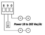
UL 61010-1 requires a 250 mA slow-blow fuse for power > 50 Vac/dc, or a 400 mA slow-blow fuse for power < 50 Vac/dc.
