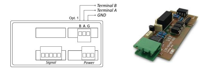
The optional S1 module provides an isolated Modbus RTU serial output. It is installed in Slot 1 and plugs directly into the display board. With only a single function (4 = read register), it is very easy to use.
