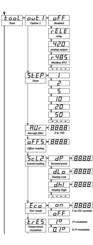
The Tools (tooL) menu is used to configure the meter.
