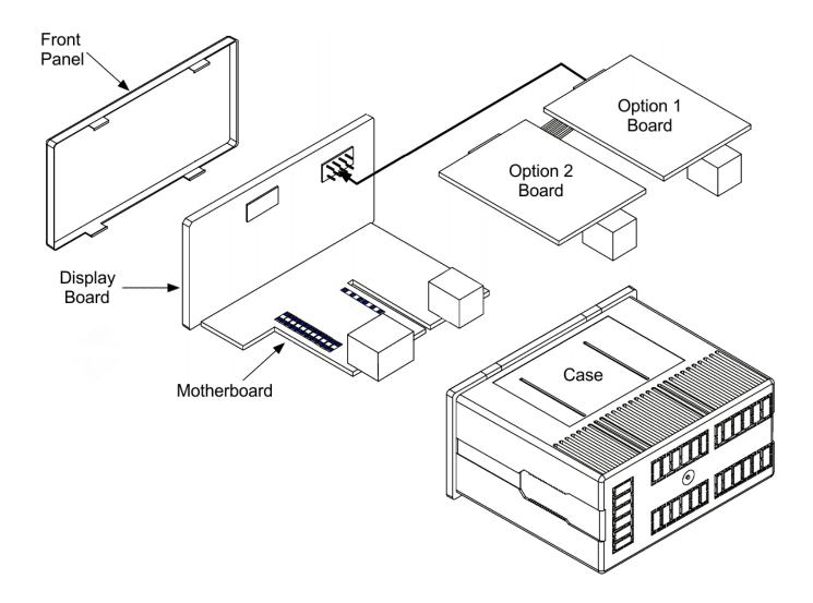
**An Electronics Main Assembly** is standard. It consists of a large horizontal Motherboard, which includes a Universal Power supply for 18-265 Vac/dc, and which performs signal conditioning and processing for all selectable signal types. Soldered to the Motherboard is a vertical Display Board, which holds the meter's LEDs and pushbuttons.
