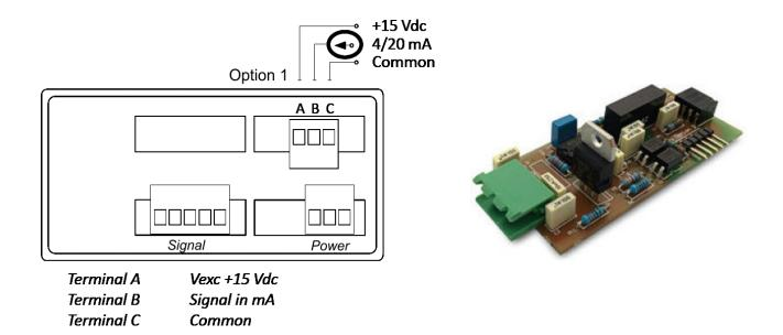
The optional M1 module provides an isolated 4-20 mA analog output. It is installed in Option Slot 1 and plugs into the display board. The 4-20 mA signal is scalable with either a positive or negative slope, and is proportional to the reading of the instrument. A sourcing mode, where the modules powers the loop, or a passive sinking mode, where an external supply powers the loop, are selectable at the connector.
