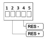
**Scaling:** The measured resistance can be scaled for readings from -1999 to 9999 with a selectable decimal point.
