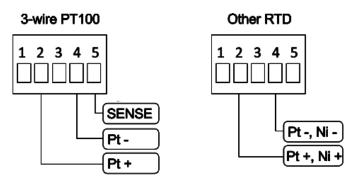
**Provision for lead wire resistance:** A 3-wire connection is jumper selectable with Pt100 RTDs to subtract lead wire resistance. If a 2-wire connection is used, the instrument allows a fixed number of counts to be subtracted from the resistance reading. This is done with the programmable "oPFFS" offset parameter.
