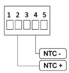
**NTC probe types:** To see if the L40 is compatible with specific NTC thermistor type, check the thermistor data sheet and note the parameters  $R_{25}$  and Beta. The instrument can be programmed for Beta values from 2000 to 5500 and accommodates resistances from 100 P to 100 kP.
