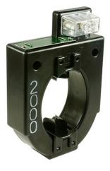
Cast units are molded in polyurethane resin and have slightly larger dimensions. The core is made from high quality grain-oriented silicon steel while the secondary winding is made from heavy enameled copper wire evenly distributed around the core for maximum accuracy and resistance to stray magnetic fields.
